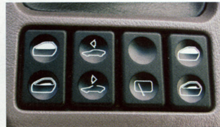
Window, rear wiper and sunroof switches are console-mounted, between armrest and shifter.
