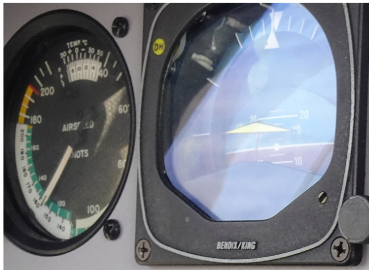
Loss of airspeed, down to 135 kts (left gauge indicated above the green band .. 155 mph/250 kph) with a climbing attitude (indicated in the right instrument).
