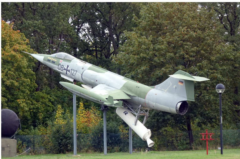
F104 with JATO ... a VERY brave pilot was needed for this ride.
